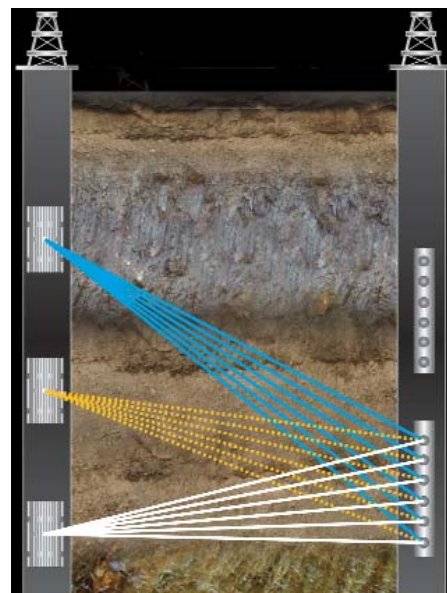
Figure 1. Soundwaves are transmitted from sources to receivers in the crosswell process. (Images courtesy of Z-Seis)
